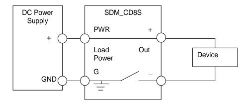
Figure 3. Typical Wiring Application
